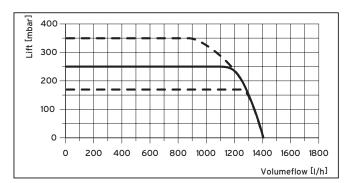
Fig. 3.11 Pump specifications ecoTEC pro
