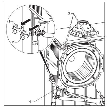
Fig. 9.5 Replacing primary heat exchanger
