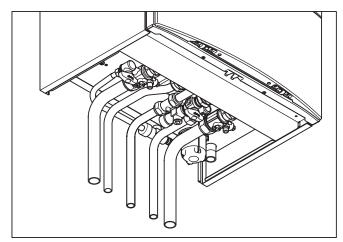
Fig. 5.3 Double check valve detached while heating
