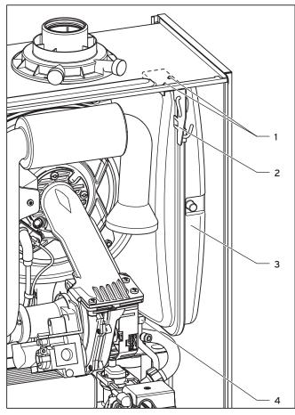
Fig. 9.4 Replacing expansion vessel
