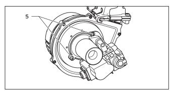
Fig. 9.3 Gas fitting/fan screwed joint
