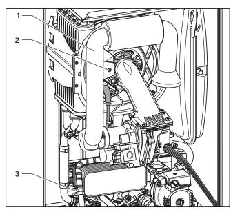
Fig. 7.1 Dismantling air intake pipe
