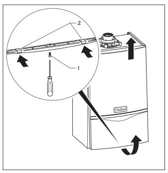
Fig. 4.4 Removing/fixing the front case
