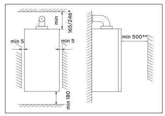
Fig. 4.1 Distances during installation (dimensions in mm)
