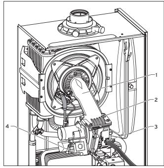
Fig. 9.2 Dismantling fan with gas fitting
