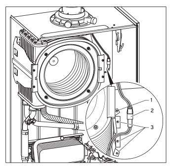
Fig. 9.6 Primary heat exchanger holder
