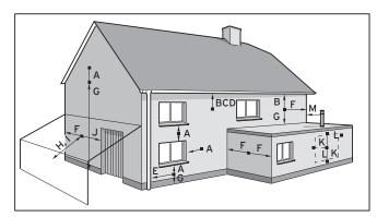
Fig. 3.8 Flue termination
