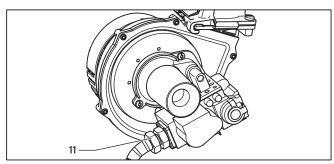
Fig. 7.8 Testing the gas supply for soundness
