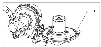
Fig. 7.5 Replacing the burner door seal
