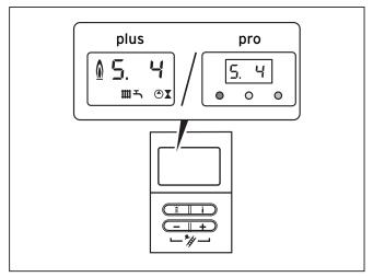
Fig. 6.2 Display indicator during heating mode
