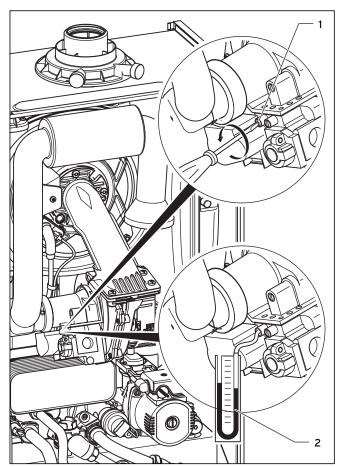
Fig. 5.13 Checking the gas supply pressure
