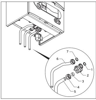
Fig. 4.7 Installing the hot and cold water connection (ecoTEC pro combination boiler)
