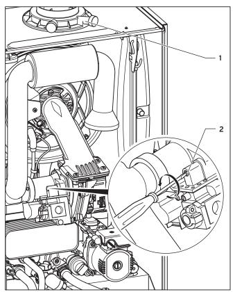
Fig. 9.7 Carrying out measurement of CO<sub>2</sub> levels, preparing for air-ratio adjustment
