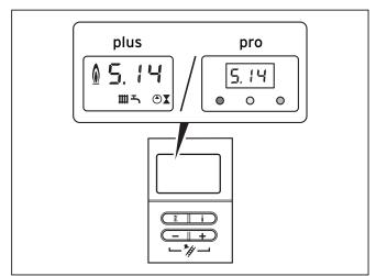
Fig. 6.3 Display indicator during water heating
