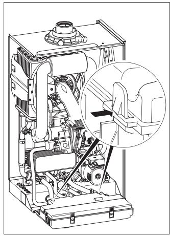
Fig. 4.13 Opening the electronics box
