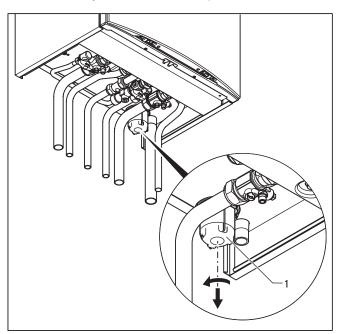
Fig. 7.9 Cleaning the condensate siphon
