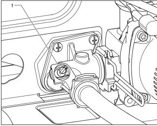
Fig. 5.12 Adjusting the by-pass valve (in system boilers)
