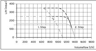
Fig. 3.10 Pump specifications ecoTEC plus
