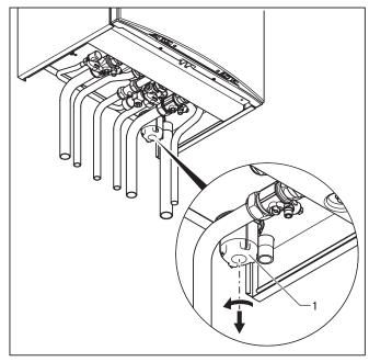
Fig. 5.4 Filling the condensate siphon
