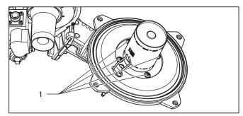
Fig. 9.1 Replacing burner
