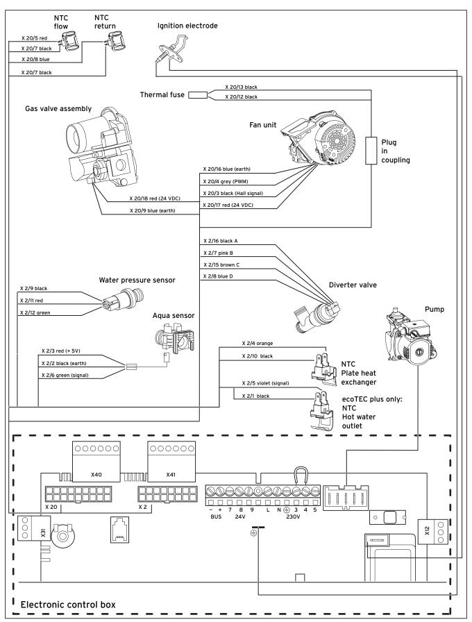
Fig. 4.16 Connection wiring ecoTEC combination boiler
