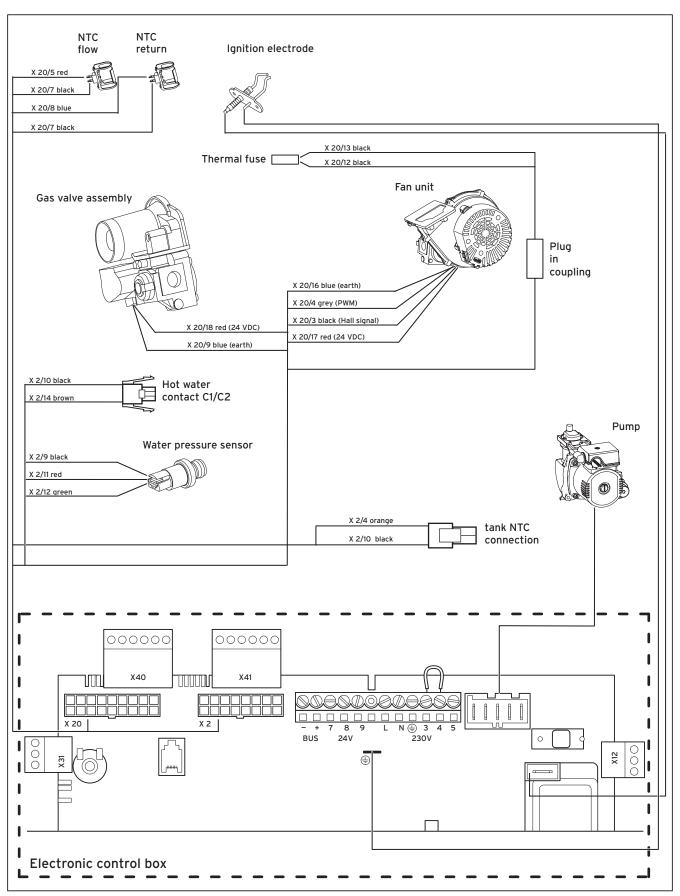
Fig. 4.17 Connection wiring ecoTEC system boiler
