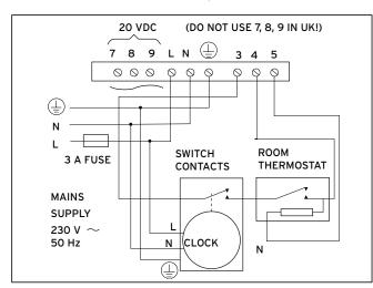
Fig. 4.18 Connection details for time switches
