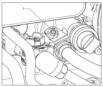
Fig. 5.11 Adjusting the by-pass valve (in combination boilers)
