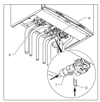
Fig. 5.2 Filling device ecoTEC plus combination boiler
