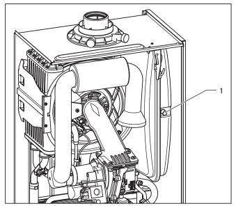
Fig. 7.10 Checking expansion vessel admission pressure
