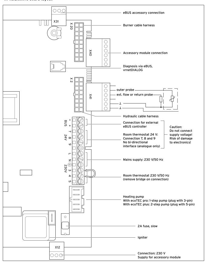
Fig. 4.15 Connection wiring ecoTEC
