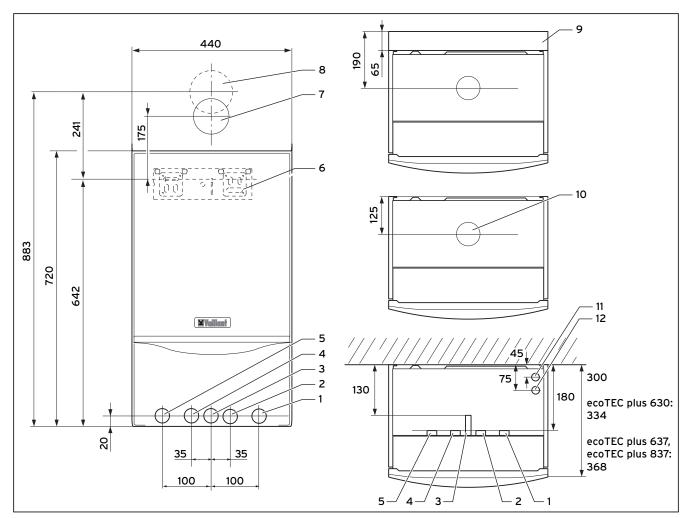
Fig. 2.1 Dimensions in mm
