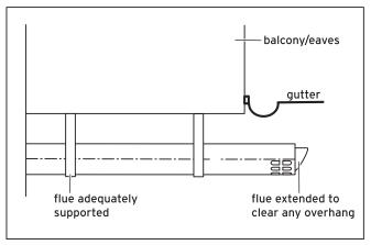
Fig. 3.9 Flue termination under balcony/eaves
