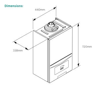
**Note:** A 500mm front clearance is recommended to allow easy access during inspection and maintenance
