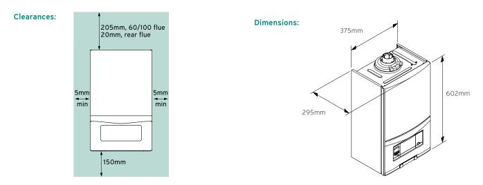
Note: A minimum of 600mm clearance in front of the boiler is required to enable easy access for servicing. This can be reduced to 5mm if fitted behind removable door/panel.
