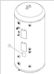
You can find the serial number on the identification plate (1), which is located on the cylinder below the electronics box.
