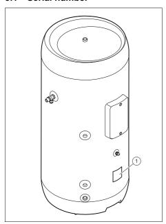
You can find the serial number on the data plate (1), which is located on the cylinder below the electronics box.
