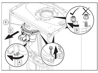
9. Remove the gas-air mixture unit (6).
