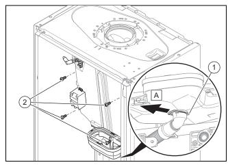
11. Remove the clip underneath the condensate tray (1).
