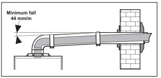
Standard flue terminal kits have an in-built fall back to the boiler to drain the condensate. These can be fitted level between the appliance and the termination position. All other extended flues must have a fall of at least 44 mm/m.
