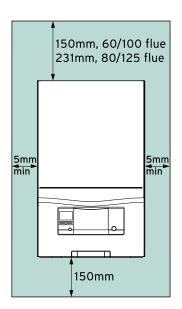
**Note:** A 600mm front clearance is recommended to allow easy access during inspection and maintenance
