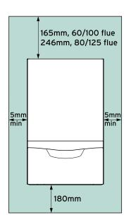
**Note:** A 500mm front clearance is recommended to allow easy access during inspection and maintenance
