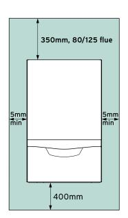
**Note:** A 500mm front clearance is recommended to allow easy access during inspection and maintenance
