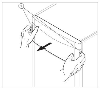
Remove the front flap on the control panel by taking hold of the recessed handles with both hands and lifting off the front flap towards you.
