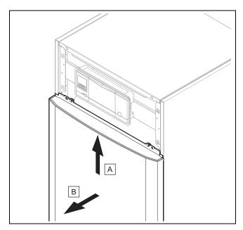
3. Pull each part of the front casing forwards slightly and remove it by lifting it upwards.
