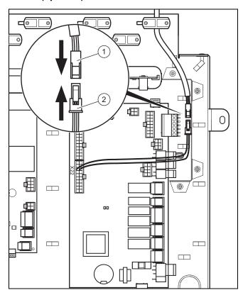
Connect the cable for the cylinder temperature sensor, which is available as an accessory, to the bush (1) on the plug (2). Use a strain relief which does not have a power supply cable running through it.
