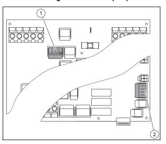
A changeover contact connection X143 (1) with the assignment Lb, La, N, PE is provided for connecting a cut-off relay for the external well pump.
