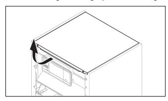
1. Pull the casing top forwards slightly and remove it by lifting it upwards.
