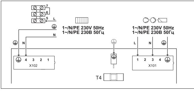
1 Power supply for internal electric back-up heater X101 Mains connection for compressor
