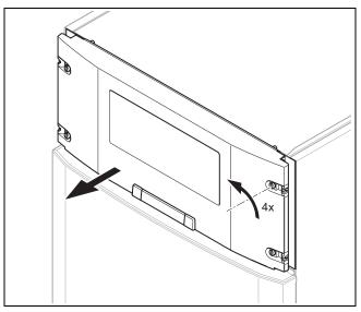
2. Turn the four screws by a quarter turn and lift off the cover on the control panel towards you.
