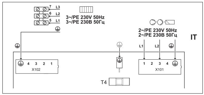
Blockable power supply for internal electric back-up heater
