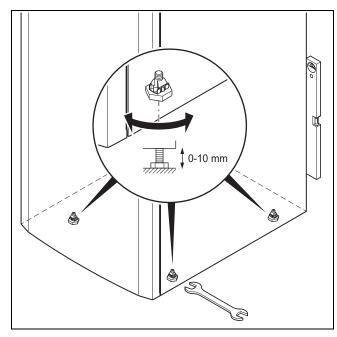
Orientate the product horizontally by adjusting the adjustable feet.
