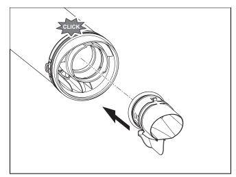
6. Slide the end pipe onto the terminal piece until you hear the end pipe click into place.
