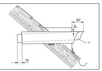
► Insert the air/flue pipe (1) into the dormer.
