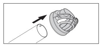
6. Pull the opening piece from the flue pipe.
