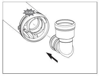
2. Slide the connection elbow onto the terminal piece until you hear it click into place.
