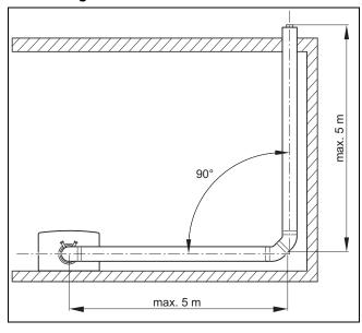
Install an 87° elbow at an angle of 3° between the wall and the air/flue pipework or use two 45° elbows. Connect all of the pipe joints with air pipe clamps.
