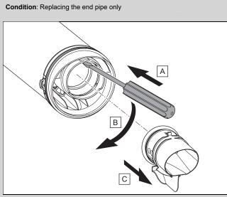
Undo the end pipe's lock (1) using a flat-blade screwdriver and pull it out to the front.
