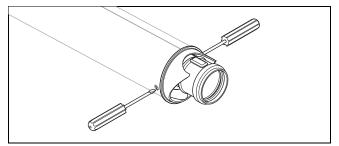
3. Use an 8 mm screwdriver to press the latching lugs inwards.
