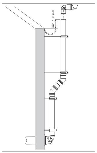
When installing the variable terminal set around eaves, additional M8 threaded rods are required for the pipe clamps. The threaded rods are commercially available.
