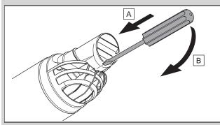
Release the catch between the terminal piece and the end pipe.
