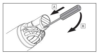
1. Release the catch between the opening piece and the end pipe.
