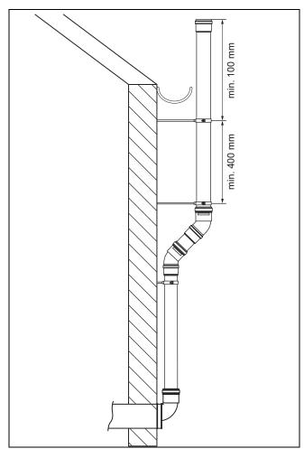
When installing the variable terminal set around eaves, additional M8 threaded rods are required for the pipe clamps. The threaded rods are commercially available.
