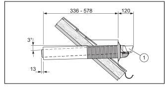
▶ Insert the air/flue pipe (1) into the dormer.
