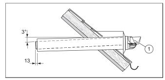
Insert the air/flue pipe (1) into the dormer.
