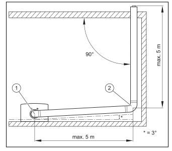
➤ To ensure that you can guide a second 87° elbow (2) at a right angle through the wall, install the elbow (1) on the top of the boiler, at a 3° rotation.
