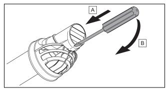
3. Release the catch between the opening piece and the end pipe.
