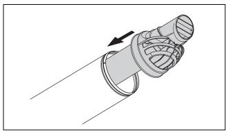
9. Slide the flue pipe with the new terminal into the air pipe until you hear the terminal click into place.
