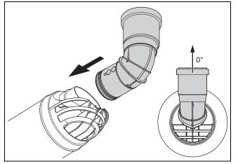
3. Slide the first 87° elbow onto the opening piece until you hear the 87° elbow click into place.
