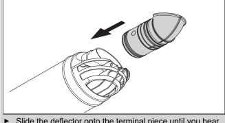
Slide the deflector onto the terminal piece until you hear the deflector click into place.
