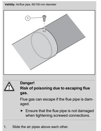
2. Use the locking screws (1) to screw the air pipes.
