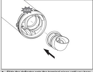
Slide the deflector onto the terminal piece until you hear the deflector click into place.
