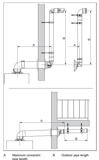
4.4.3 Maximum pipe length for vertical roof duct
