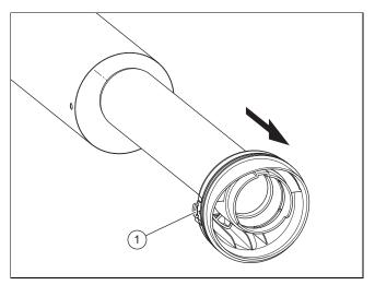
2. Pry open the snap-on connections (1) on both sides using a flat-blade screwdriver and use the terminal piece to pull the flue pipe out of the air pipe.
