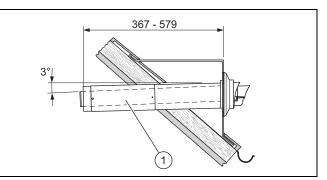
Install the roof duct in the dormer in the same way as the wall duct (→ Section 5.11.2).
