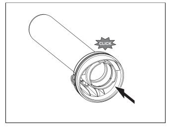
4. Slide the new terminal piece onto the flue pipe until you hear the terminal piece click into place.
