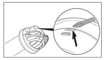
5. Release the catch between the opening piece and the flue pipe.
