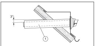
Install the roof duct in the dormer in the same way as the wall duct (→ Section 5.10.3).
