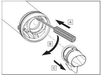
1. Undo the end pipe's lock using a flat-blade screwdriver and pull it out to the front.
