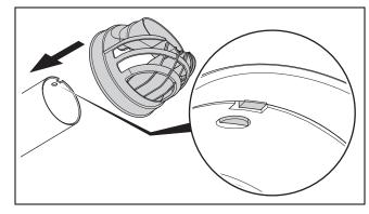
7. Slide the new opening piece onto the flue pipe until you hear the opening piece click into place.
