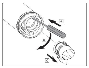
1. Undo the end pipe's lock using a flat-blade screwdriver and pull it out to the front.
