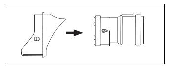
7. Pull the terminal piece out of the pipe adapter.
