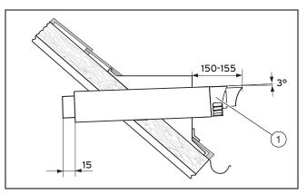
Insert the air/flue pipe (1) into the dormer.
