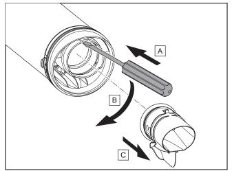
Undo the end pipe's lock using a flat-blade screwdriver 1. and pull it out to the front.
