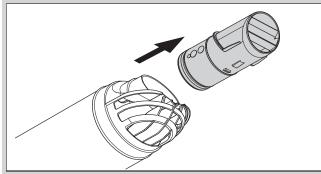
Pull the end pipe from the terminal piece.
