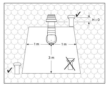
Extremely damp extract air escapes from the channel vents. This may condense in the air pipe and cause damage to the product.
