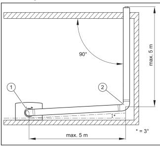
► To ensure that you can guide a second 87° elbow (2) at a right angle through the wall, install the elbow (1) on the top of the boiler, at a 3° rotation.
