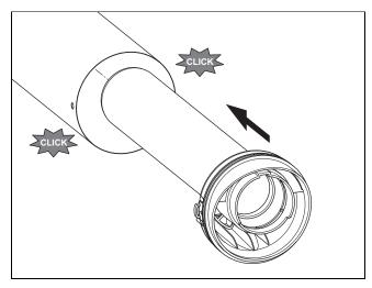
5. Slide the flue pipe with the new terminal piece into the air pipe until you hear the terminal piece click into place.
