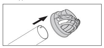
6. Pull the opening piece from the flue pipe.
