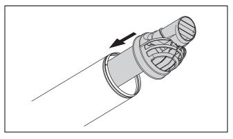
9. Slide the flue pipe with the new terminal into the air pipe until you hear the terminal click into place.
