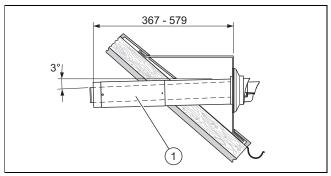
Install the roof duct in the dormer in the same way as the wall duct (→ Section 5.11.2).
