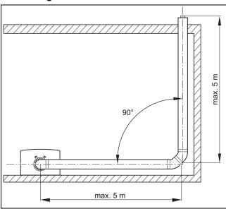
► Install an 87° elbow at an angle of 3° between the wall and the air/flue pipework or use two 45° elbows.
