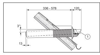
▶ Insert the air/flue pipe (1) into the dormer.
