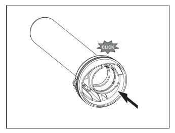
4. Slide the new terminal piece onto the flue pipe until you hear the terminal piece click into place.
