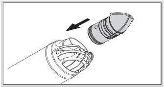
Slide the deflector onto the terminal piece until you hear the deflector click into place.
