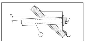
► Install the roof duct in the dormer in the same way as the wall duct (→ Section 5.10.3).
