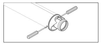
Use an 8 mm screwdriver to press the latching lugs inwards.
