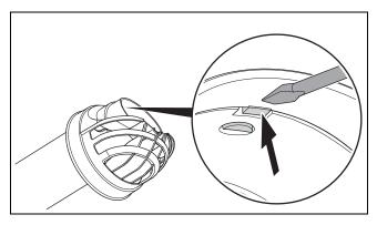
5. Release the catch between the opening piece and the flue pipe.
