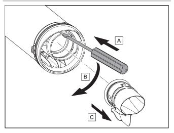
Undo the end pipe's lock using a flat-blade screwdriver 1. and pull it out to the front.
