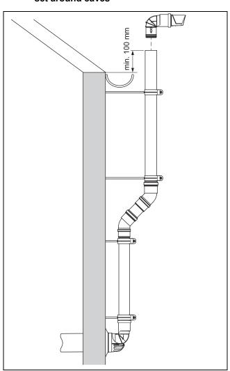
When installing the variable terminal set around eaves, additional M8 threaded rods are required for the pipe clamps. The threaded rods are commercially available.
