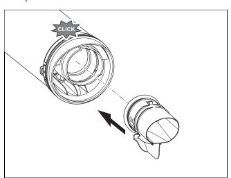
6. Slide the end pipe onto the terminal piece until you hear the end pipe click into place.
