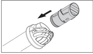
8. Slide the end pipe onto the opening piece until you hear the end pipe click into place.
