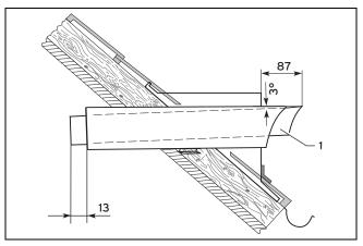
Insert the air/flue pipe (1) into the dormer.
