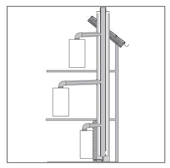
Markings have been assigned to the air/flue system in accordance with EN 1443 and these indicate that the system complies with the fundamental requirements of the construction products directive. The air/flue system is not approved as part of the boiler.
