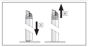
1. Detach the terminal with the flue pipe by pushing the air pipe to the floor.
