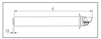
2. Shorten the flue pipe and the air pipe by the same amount when they are assembled.
