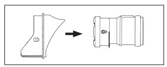
7. Pull the terminal piece out of the pipe adapter.
