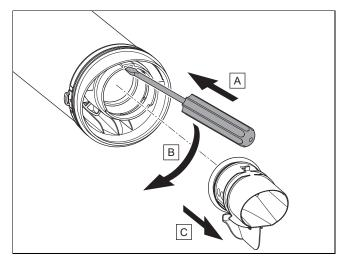
Undo the end pipe's lock using a flat-blade screwdriver and pull it out to the front.
