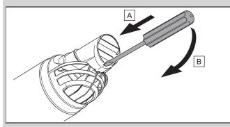
Release the catch between the terminal piece and the end pipe.
