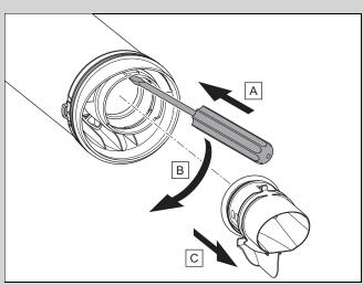
Undo the end pipe's lock (1) using a flat-blade screwdriver and pull it out to the front.
