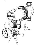
VaillantUK vaillantuk VaillantUK vaillant.uk Vaillant UK A - Pressure Gauge: The pressure Gauge is rated to Max ABar, if over pressure is encountered Drain point (E) can be opened to allow water safely out of the system via a hose, to a bucket or drain. This can be operated with a standard radiator bleed key.
