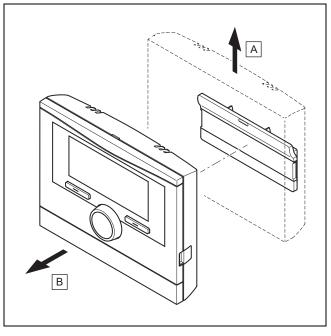
1. Remove the system control from the unit mounting bracket as shown in the figure.
