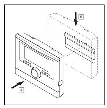
Clip the system control into the unit mounting bracket as shown in the figure, making sure that it clicks into place.
