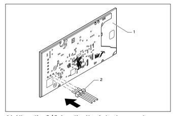
4.1 Alternative 2/2: Inserting the pin header connector horizontally
